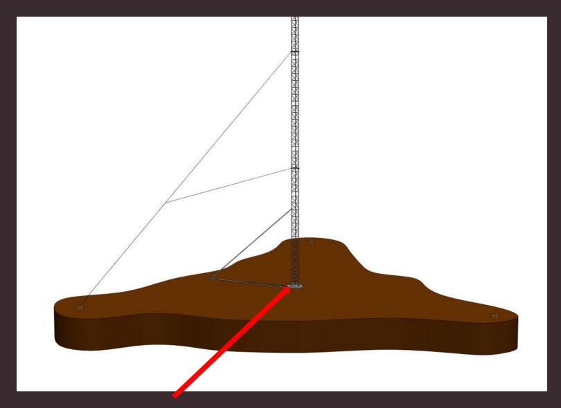
When lift is complete, insert the M16 base hinge bolt and fasten all base bolts securely. Attach the anchor cables to the anchors securely before removing the lifting cable or climbing the tower.
