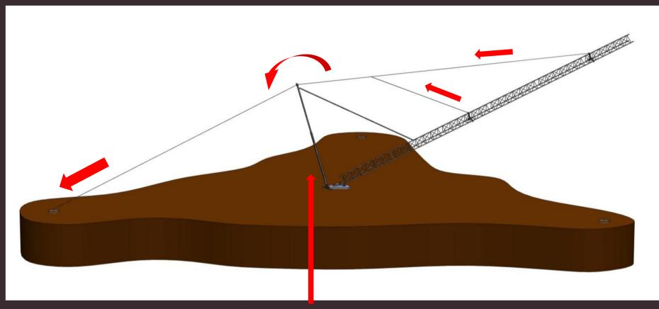
Note that the lifting pole moves synchronously with the tower and should remain perpendicular to the tower during the lift.
