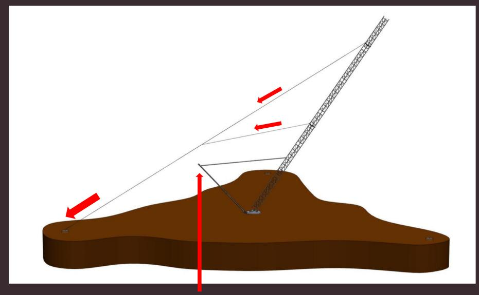
Note that the lifting cable separates from the lifting pole once lever angle is crossed but the lifting pole will continue to move in sync with the tower.
