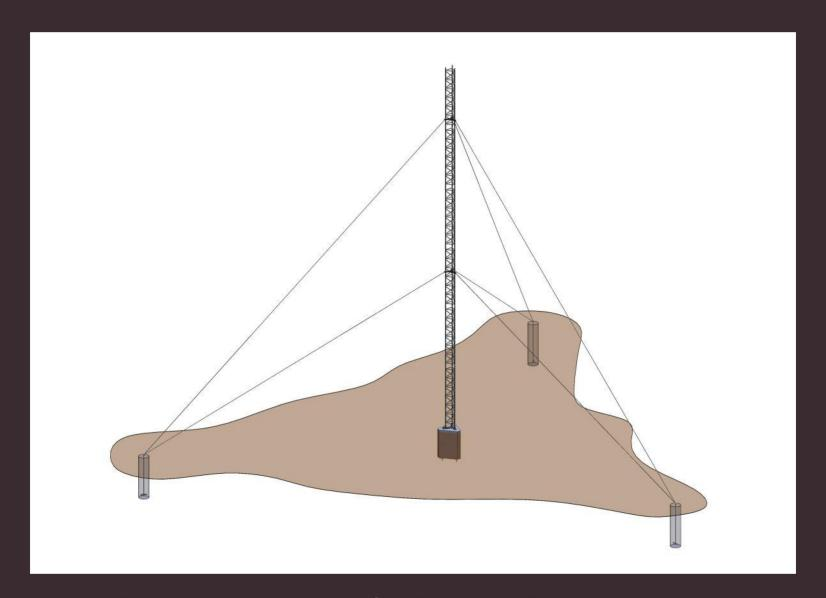
Ensure all guy cables are evenly tensioned. Should the tower be off plumb, the guy cables along with the t-base anchor nuts can be used to straighten the tower but ensure that the guy cables are evenly loaded.
