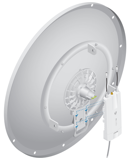
AF-5XHD Mounting onto RocketDish RD-5G30
