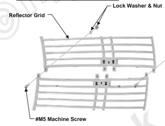
Assemble the halves of the Reflector Grid using (2) #M5 machine screws with lock washers, flat washers and nuts as shown.
