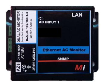
Our Site – Monitor products permit the monitoring and control of equipment at any site with IP connectivity in the comfort of your office. **The Ethernet Relay + e-MAIL** is the perfect addition to any remote repeater site to control and monitor equipment remotely via Ethernet, email and SNMP.
