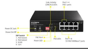
Long Range 8-Port Gigabit Switch with 4 PoE+ Ports & DIP Switch
