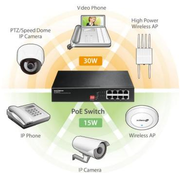
\*IP Phone: 3- 7W, IP Camera: 7- 10W PZT Camera: 15 -25+ W
