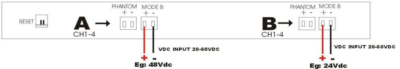
**POWER Connection - PHANTOM for POE A + POE B at the same voltage**
