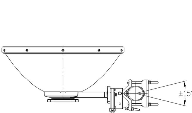
Fine Azimuth Adjustment
