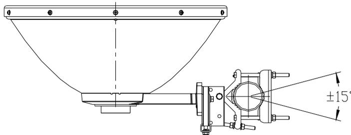
Fine Azimuth Adjustment
