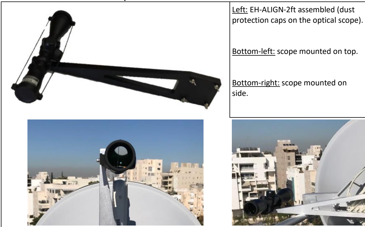
FIGURE 2: Assembled scope mounted on 2ft antenna
